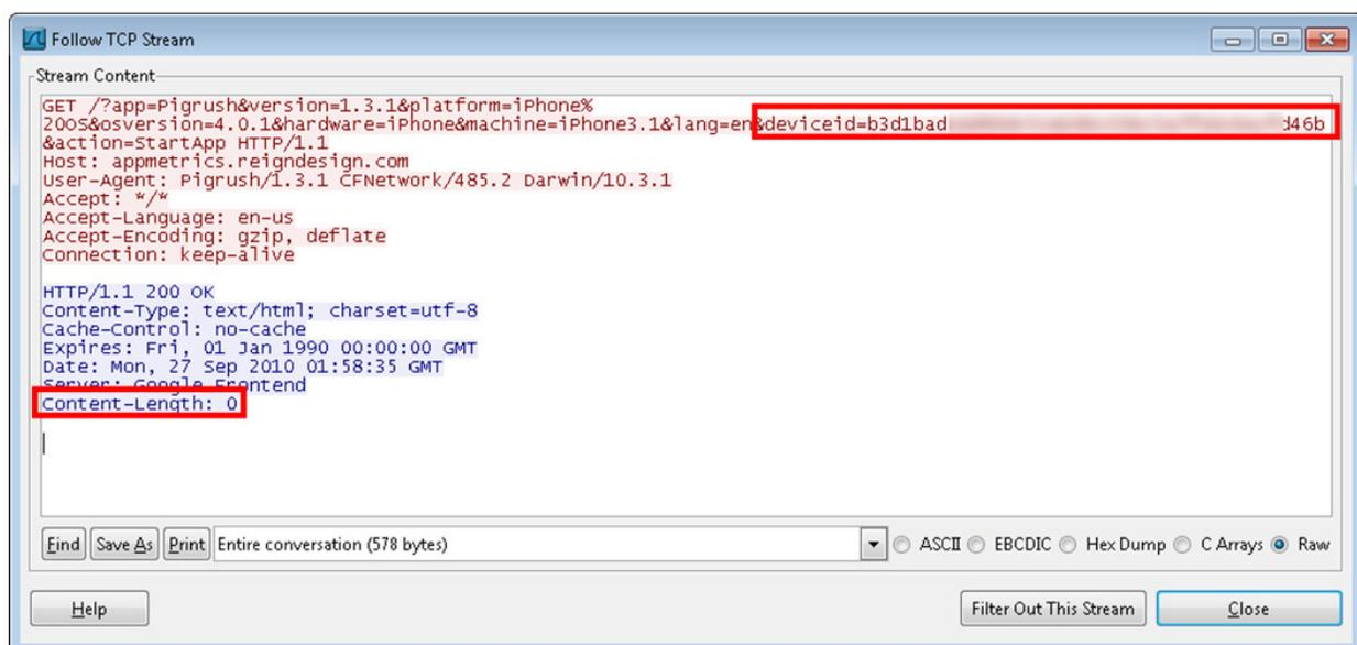
**Figure 3: A typical UDID tracking conversation between an application and a remote server. Note the size of the response message at zero bytes, indicating that this communication was initiated by the application strictly for tracking purposes, and not to retrieve any sort of remote content.**
